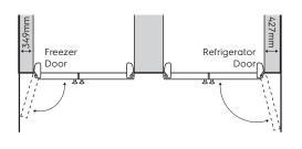
Make sure that cupboards or fi xtures do not stick out further than the refrigerator.
